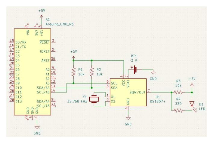
Note that the backup supply is a 3V coin cell. This supply will allow the DS1307 to keep track of time when it is turned off.
