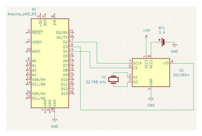
Note that the backup supply is a 3V coin cell. This supply will allow the DS1302 to keep track of time when it is turned off.
