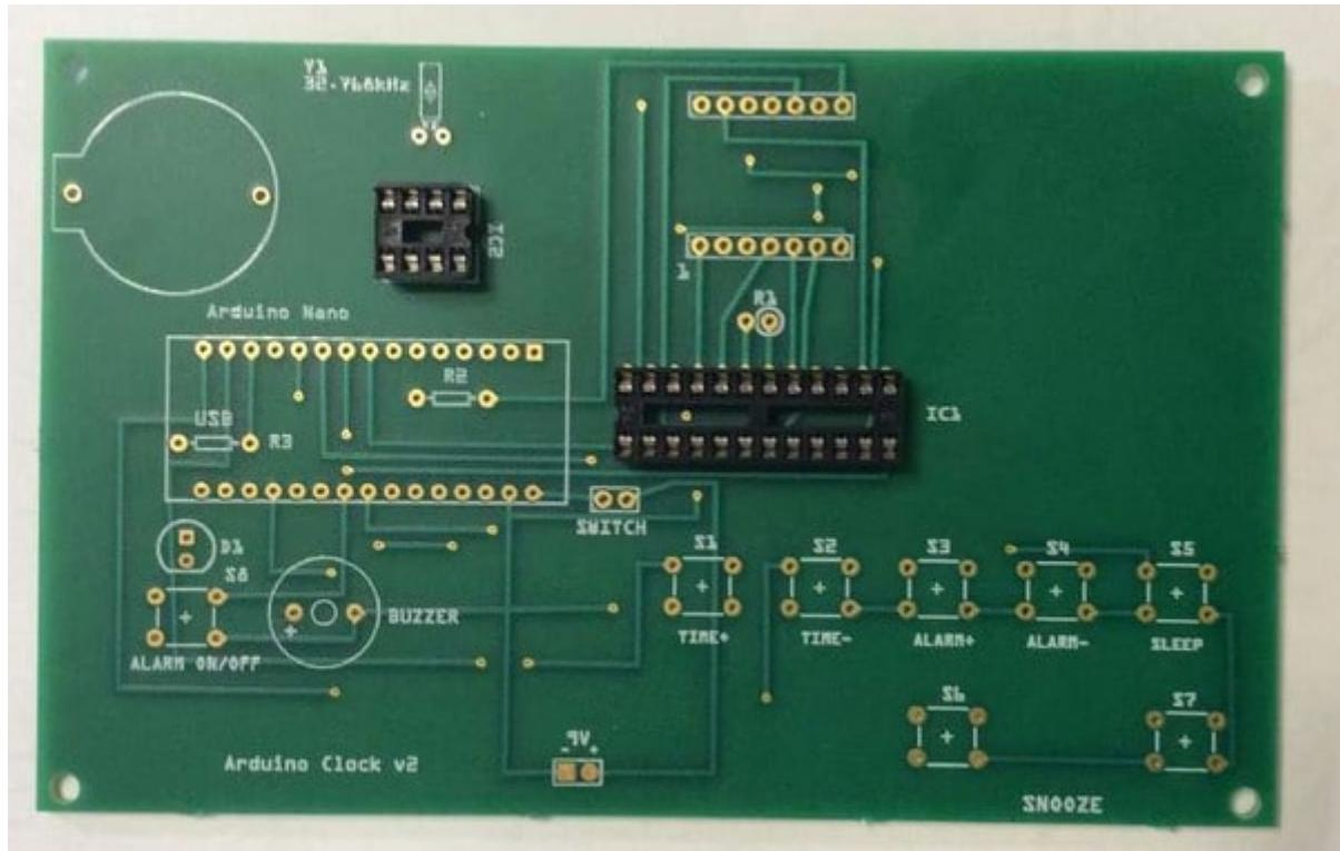
2. Solder on both rounded female headers (7 pins).
