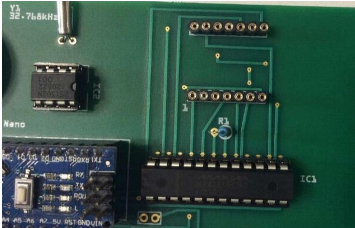
12. Note the small "1" on the PCB. This indicates where pin 1 of the display should be connected. Insert the display into the rounded female headers. Then, insert a 3V coin cell into the coin cell holder. The side marked with a "+" should be on top.
