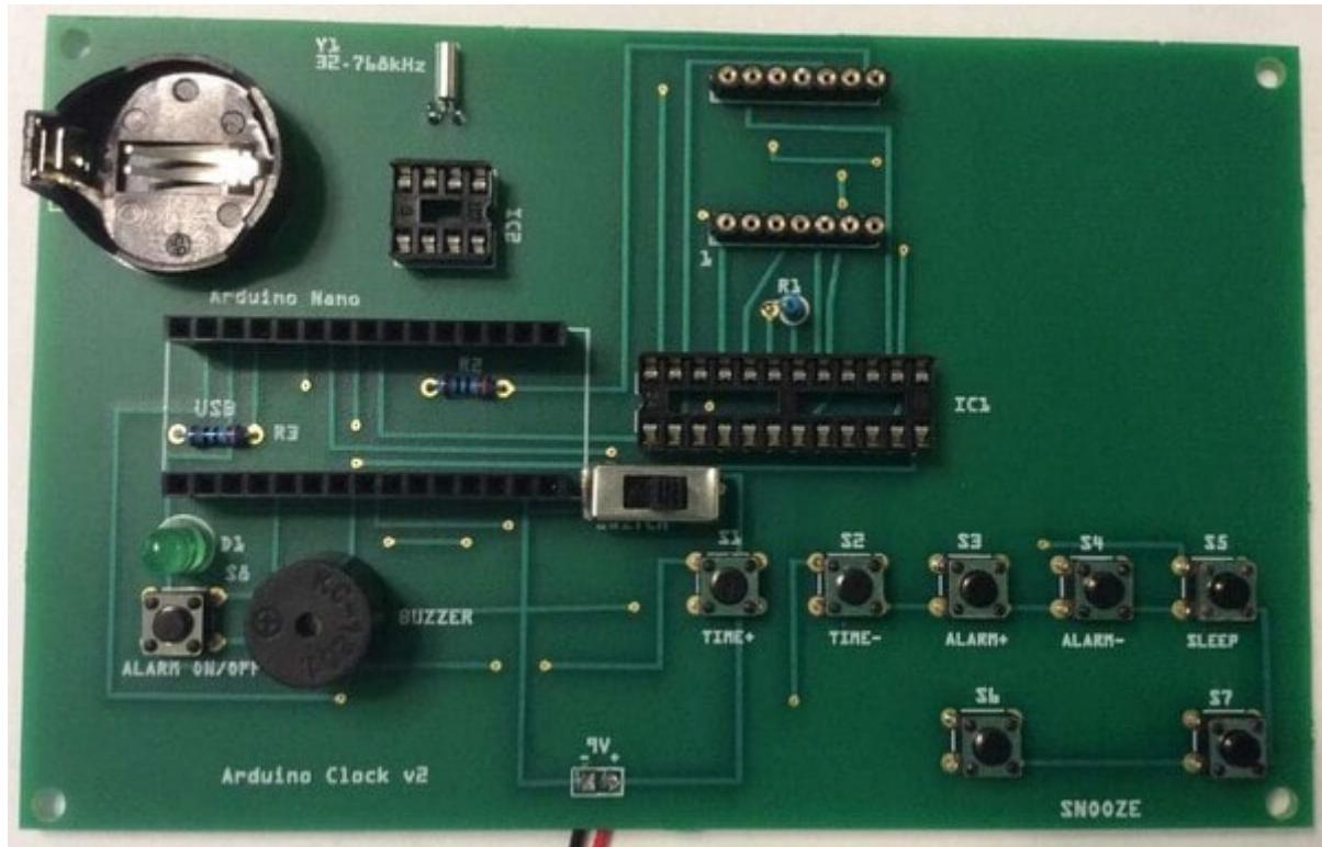
10. Bend Y1 downward. Then, insert the Arduino Nano into the two long female headers. The USB port should be over the word "USB" on the PCB.
