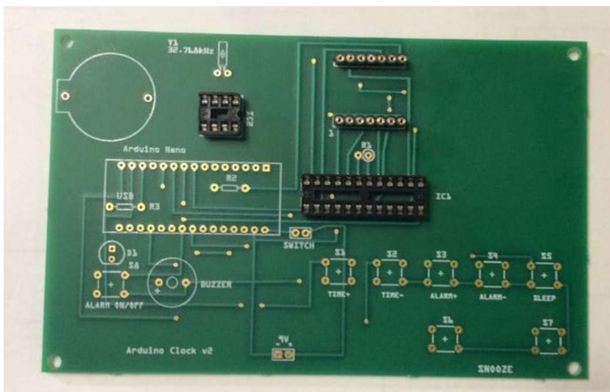
3. Solder on the battery holder, R2, and R3 (both 220R).
