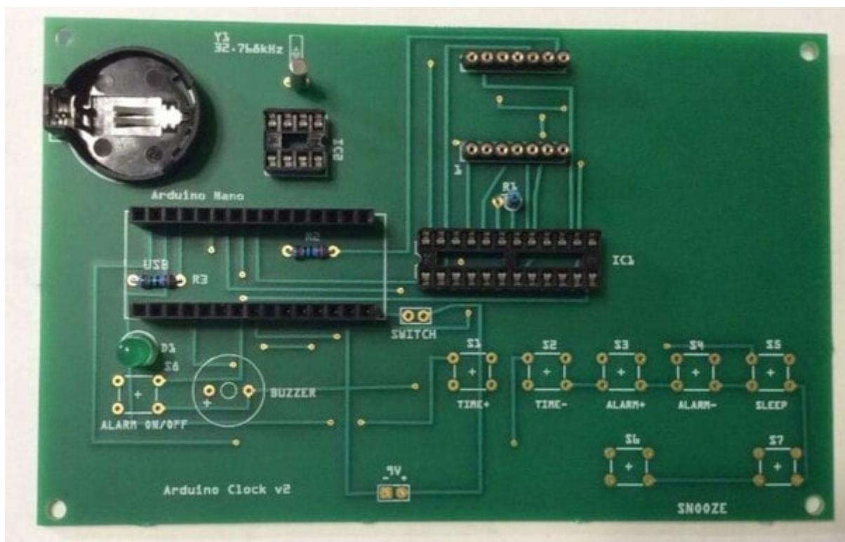
7. Solder on S1-8 and the buzzer. Make sure that the "+" on the buzzer is on the left.
