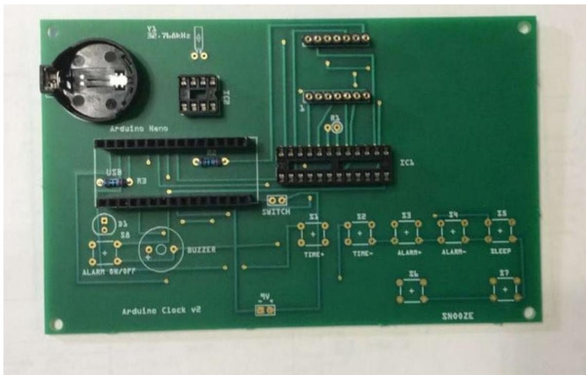
5. R1 is mounted vertically to save space. Bend one of the leads 180 degrees to make it fit. Then, put it on the PCB with the actual resistor in the circle. Next, be sure to leave at least 2mm of lead space on Y1 at the top of the PCB. Solder on R1 and Y1.
