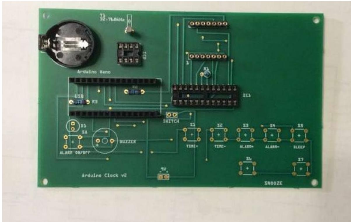
6. Solder on D1. Make sure that the anode goes into the square pad.
